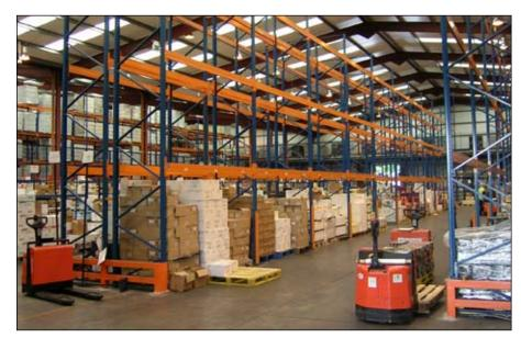
ADJUSTABLE PALLET RACKING is the most widely used storage system for all palletised and non-palletised loads. Single or double-sided runs of racking are separated by aisles that can be sized to suit the customer's forklift trucks.
