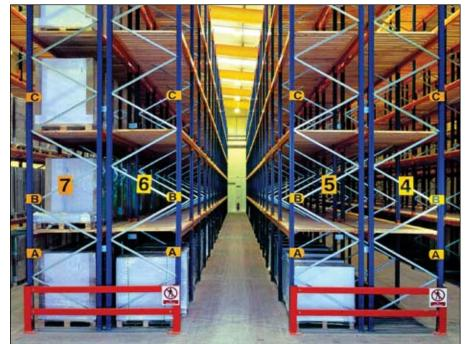
NARROW AISLE RACKING consists of Adjustable Pallet Racking but with rows installed closer together eliminating the wasted space of wide aisles. The pallets can be stored to a greater height to maximise the available headroom. The system is operated by special narrow aisle trucks, guided by floor-mounted rails or electronic wire guidance fitted in the floor.
