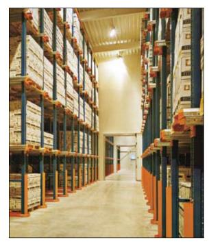
DRIVE-IN RACKING is used where high-density storage is required. It is frequently used in facilities with a low number of product lines. Pallets are stored in a block system with a reduced number of aisles. Forklifts drive into the racking to load or retrieve pallets, which are stored on cantilevered rails running throughout the system. The first pallet in is the last one out unless a Drive-Through system is used whereby pallets can be loaded or retrieved from either side.
